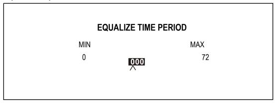
When the battery is at full voltage (not being recharged), this selection reads EQUALIZE TIME PERIOD (hrs). When the battery is recharging, this selection reads EQUALIZE TIME REMAINING (hrs). After the equalize recharge time has expired, the indication returns to the preset equalize time.
